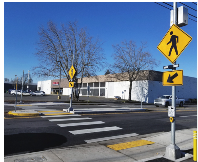
Example of a completed Rectangular Rapid Flashing Beacon (RRFB) crossing, creating a safer and more visible pedestrian crossing along a busy corridor.
